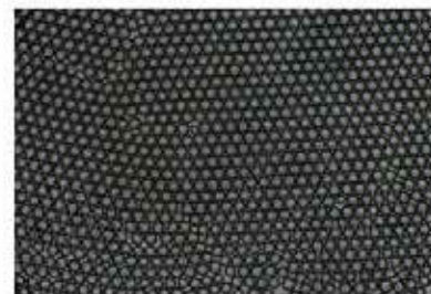
Homogenous droplets (bottom) with less than \pm 10\% variation are produced using the schematic (top).
