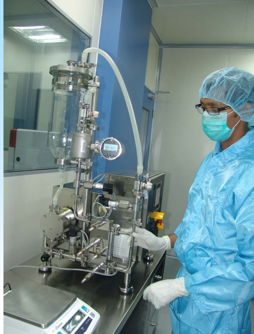
Tangential Forward Flow (TFF) system for Filtration of Protein
